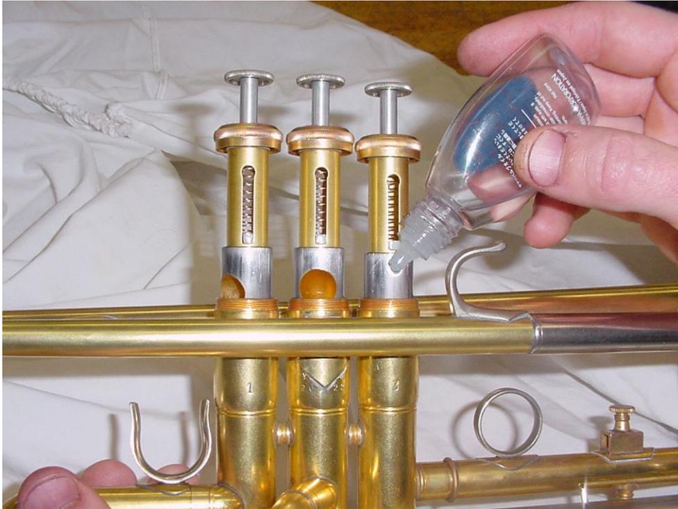
Preferred by many repair technicians and professional players. Oiling the pistons from the top to bottom offers a sheeting action which carries dirt and debris down the valve caps and offers a clean coating of oil over the entire piston surface. This properly lubricates and offers the pistons prolonged life. Note: Use 6 – 8 drops of oil per piston. Also, spinning the piston is **not** necessary to distribute the valve oil – it only serves to scratch and score the piston face.
